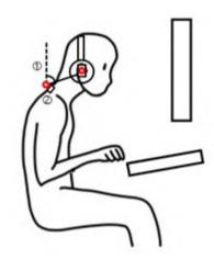
**Figure 1.** Posture during experiment (1: Definition of the neck angle, 2: Placement of the feedback System).
